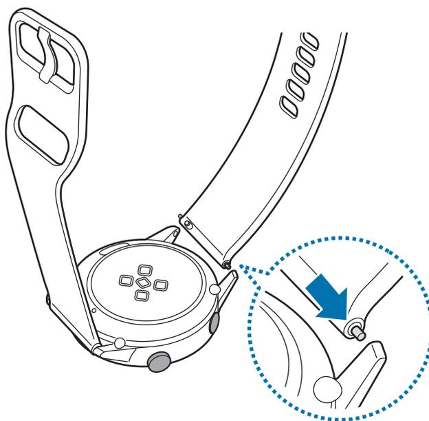
4 Slide the spring bar inwards and connect the new band.
